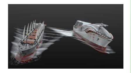
Develop and demonstrate at full scale two first-of-a-kind vessel concept designs (Kamsarmax bulk carrier and Meraviglia class cruise)
